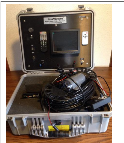
Figure 3. Video recording unit. Displays footage in real time and records to SD card.
