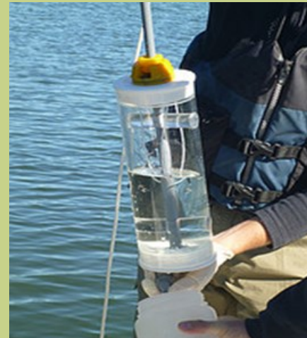
A Van Dorn style water sampler is used to collect water samples which are then transported to the lab for genetic testing.
