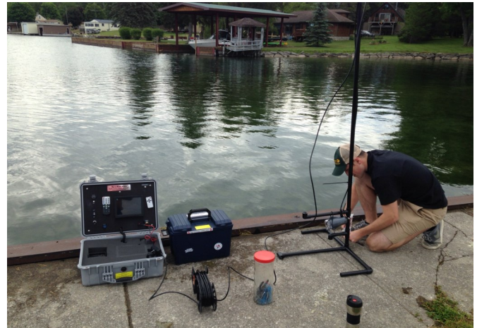
Pictured above: Nate Fedrizzi preparing a high definition, color submersible camera for video surveillance. Pictured below: Nate Fedrizzi filtering a water sample for DNA. Photo Credits, Rob Williams, SLELO PRISM.
