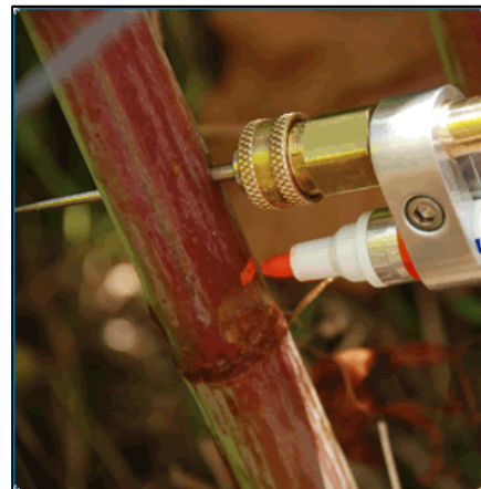
Figure 11: View of herbicide injection gun required for stem injection management of Japanese knotweed. Photo credit: JK International Injection Tools.
